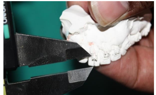
Fig. 10: Measuring the occluso-gingival height of the bonded bracket
