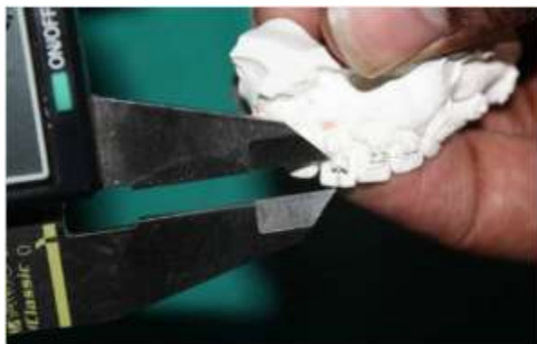
Fig. 2: Measurement of bracket positioning by using Digital Caliper
