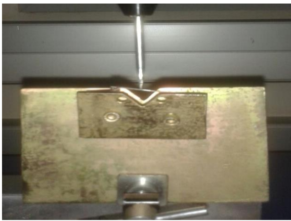
Fig. 2: Jig in the universal testing machine with unlevelled brackets
