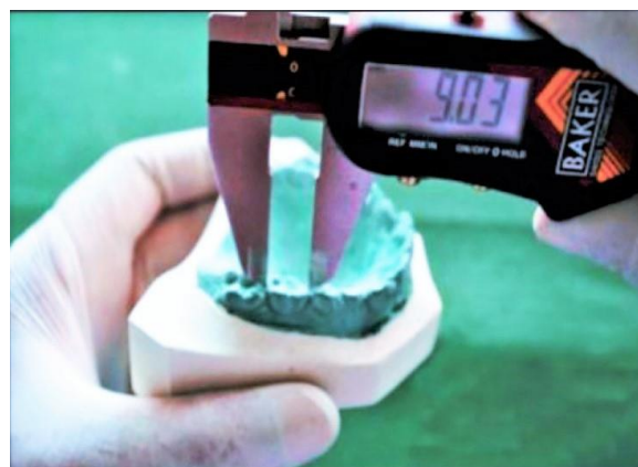
Fig. 2: Measuring teeth dimension with digital caliper
