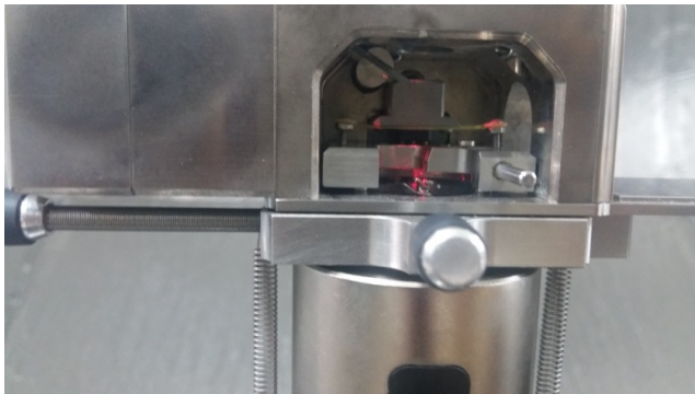
Figure 2: Bracket been scanned under atomic force microscope
