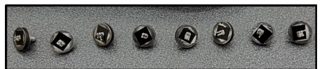
Figure 6: Loading of samples for SEM testing
