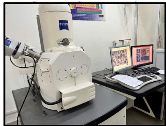
Figure 5: Setup of Scanning electron microscopy
