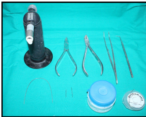
Fig. 1: Gas torch, universal plier, distal end cutter, tweezers, probe, 0.017 x 0.025 gauze S.S wire, Cut pieces of, 0.017 x 0.025 gauze S.S wire, soldering flux, soldering wire.
