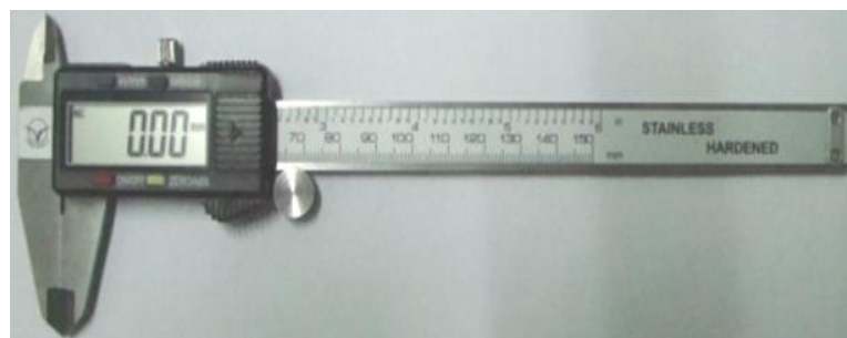
Fig. 3: Digital Vernier Calliper (Indian Aeronautics Limited)
