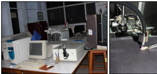
Fig. 4: a) SpectraAcq controller & set up b) Measurement of individual tooth fluorescence
