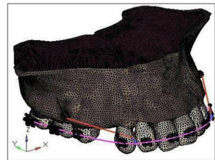
Fig. 1: Final FEM model
