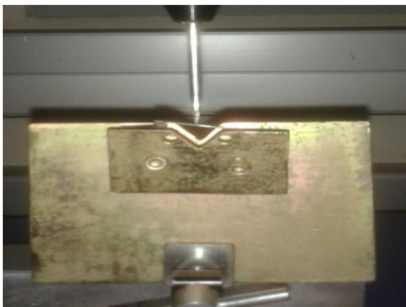
Fig. 2: Jig in the universal testing machine with unlevelled brackets
