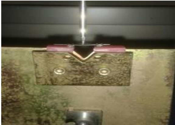
Fig. 1: Jig in the universal testing machine with levelled brackets
