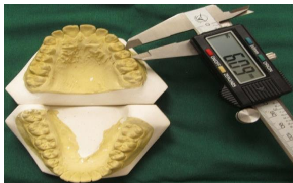
Fig.1: Digital caliper used to measure tooth dimension on study model with resolution of 0.01 mm (make-Aerospace)
