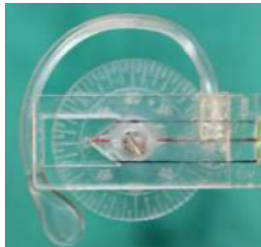
Figure 3: Round protractor with adjustment screw for angulations.
