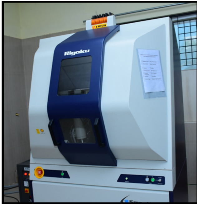
Fig. 7: Energy dispersive X-ray spectroscopy EDS (Rigaku EDS HyPix-3000)
