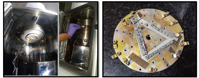
Fig. 4: RF magnetron sputtering before coating (Left) & after coating (Right).
