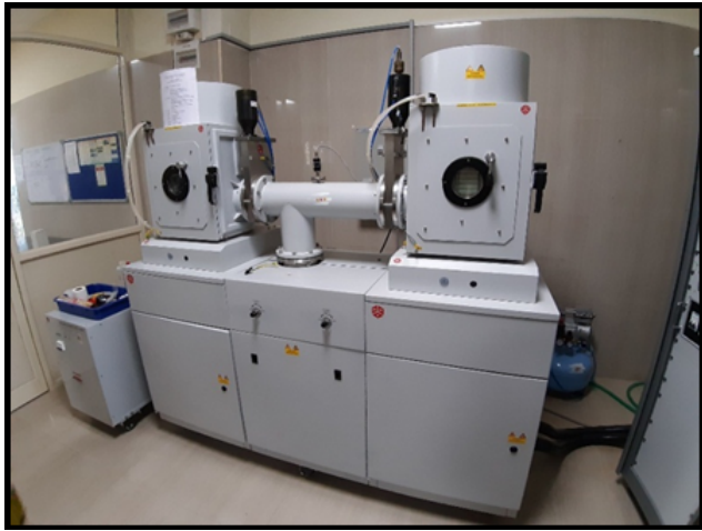
Fig. 6: RF magnetron sputtering unit HHV
