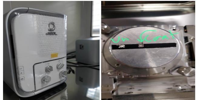
Fig. 5: Scanning electron microscope (JOEL SEM S 2200)
