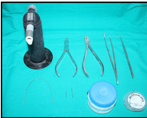
Fig. 1: Gas torch, universal plier, distal end cutter, tweezer, probe, 0.017 x 0.025 gauze S.S wire, Cut pieces of, 0.017 x 0.025 gauze S.S wire, soldering flux, soldering wire.
