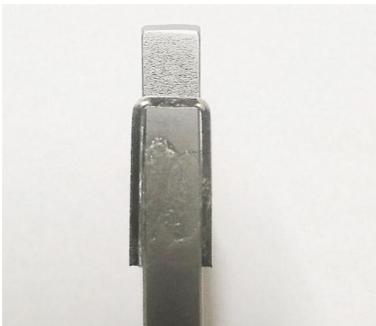
Fig. 3: The half rectangular-shaped wires are capped and glued on the measuring edges of the MBT gauge.
