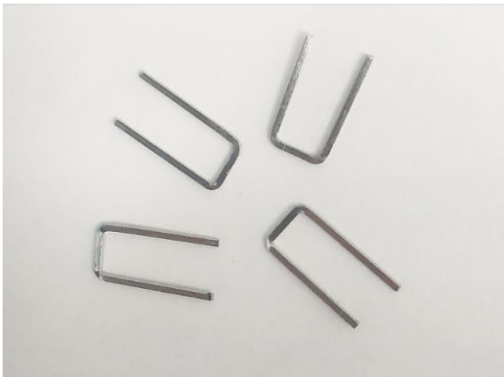
Fig. 2: Four sections of 0.021" × 0.025" SS straight wire bent in half rectangular shape.
